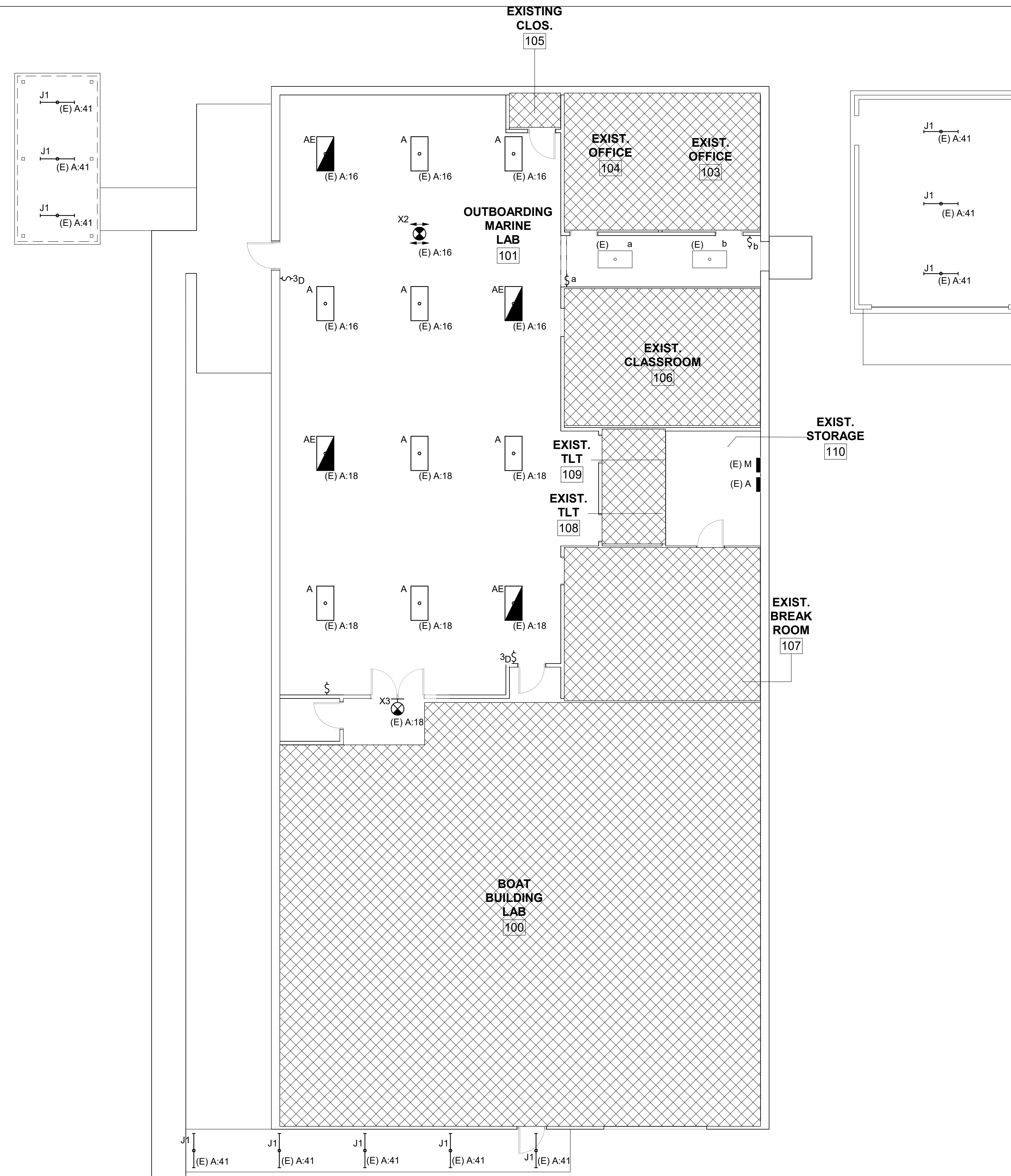
1 BUILDING 500 LIGHTING PLAN E202 SCALE: 1/8" = 1'-0"
